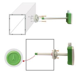
\*\*If it is a north wind and the wind will blow from north to south, the arrow should point to the south.\*\*
